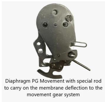
A thin corrugated membrane is built-in between the two flanges of the diaphragm pressure gauges. Pressure applied on one side of the membrane will deflect itself against the direction of the incoming pressure. This deflection of the diaphragm is a measure for the incoming pressure and is carried over to a gear segment onto the gear of the movement. This technology provides a much higher overload safety (up to 40 bar) than standard Bourdon Tube gauges.
