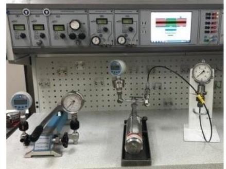
The units are displayed in PSI, kgf/cm<sup>2</sup>, bar, mbar, mmH<sub>2</sub>O, mmHg, MPa, kPa, Pa.
