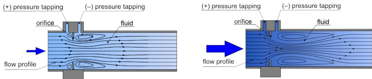
A differential pressure arises at a pipe constriction, which is proportional to the square of the flow rate through the pipe. The resulting differential pressure can be recorded with a meter and can be directly indicated as flow rate on a scale.
